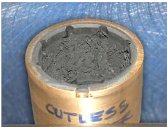
Severe wear; after 20 sec excessive vibration, black smoke & motor rpm dropped drastically.
