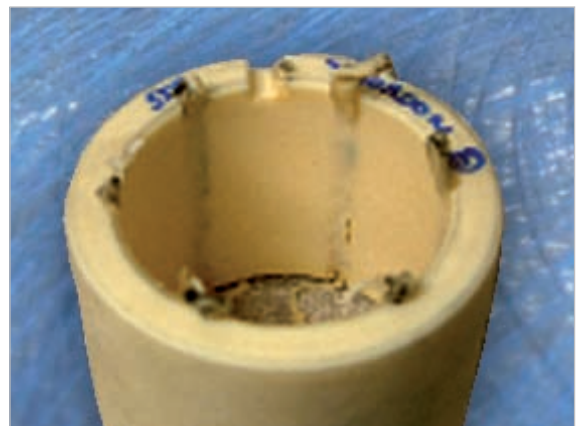
Worn cross section & inner diameter; grooves completely filled with excess material; slivers of material extruding from the grooves.
