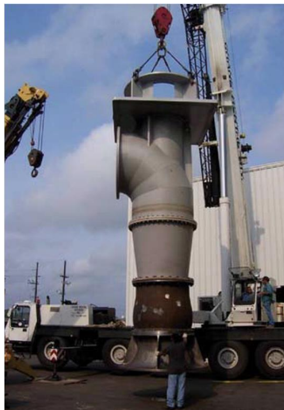
Circulating water pump
